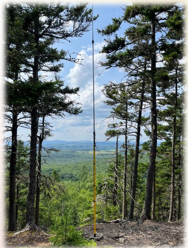
AJ1S' PODDA Pole configured as a 20m Ground Plane Vertical Aroostook State Park K-2380 (US-ME)
