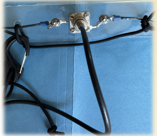
Front View of Feed Point with Dipole Leg connected and strain relief
