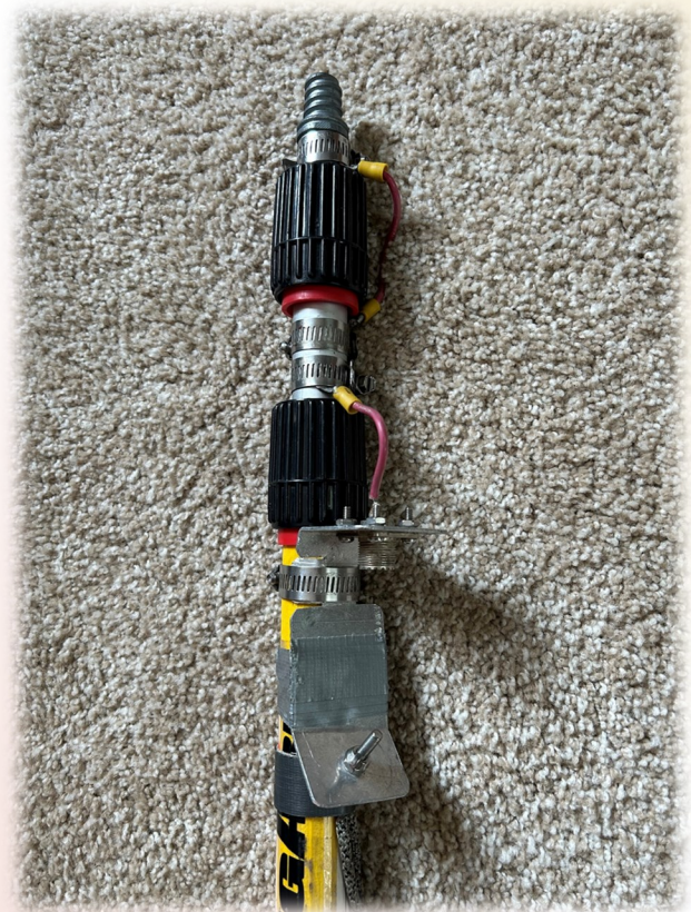
Jumper Wires to Tubes Attachment
